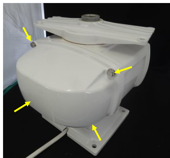
23) Attach the back cover by tightening four fixing bolts. (Tool: Wrench 13mm)
