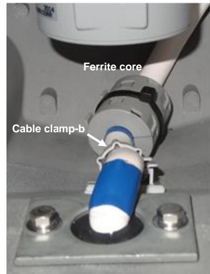
14) Clamp the cable by the cable clamp-b.
